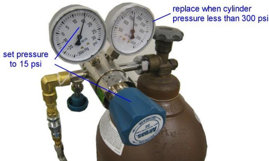
Figure 2-9 Helium gas bottle with regulator.
