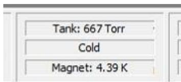
Figure 1-2. Cryostat monitor status panel showing “Cold” cryostat.
